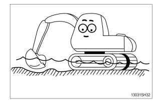
This machine has ROPS / FOG with option. Do not attempt to repair a rollover protective structure (ROPS) after an accident. Repaired structures do not provide the original structure and protection. Test and approved as a protective CAB according to ROPS and FOG standard. Meets : ISO 10262 / 3449 / 12117-2 SAE J1356 / JISO 3449
