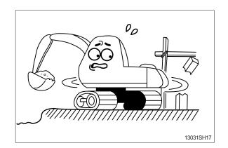
The operation on a slope is dangerous. Avoid operating the machine on a slope of over 10 degree.
