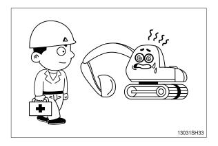
Park on a flat place and stop the engine for inspecting and repairing. Properly TAG machine is not operational. (remove start key) Extreme care shall be taken during maintenance work. Parts may require additional safe guard.
